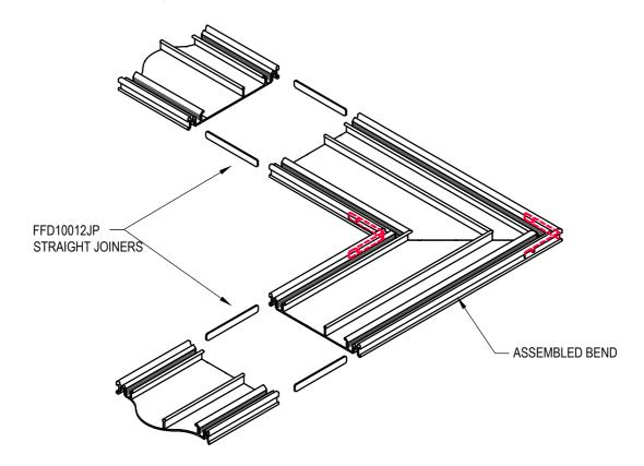
AFTER DUCT IS CABLED, FIT UNIVERSAL FLUSH COVER SET USING SCREWS PROVIDED
