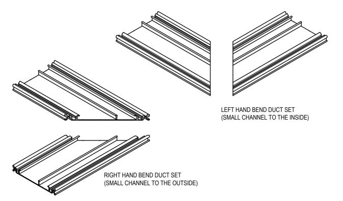
ASSEMBLE BEND DUCTS BY INSERTING 90° JOINERS & SECURING WITH SCREWS PROVIDED
