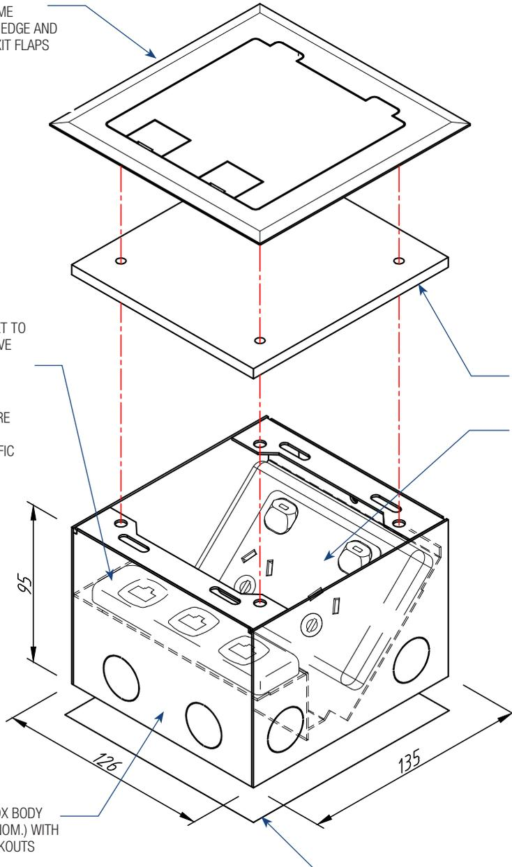
POWDER COATED STEEL BOX BODY 126 x 135 x 95 mm DEEP (NOM.) WITH 10 No. 25 $\phi$  CONDUIT KNOCKOUTS (2 EACH SIDE & 2 ON BASE)
