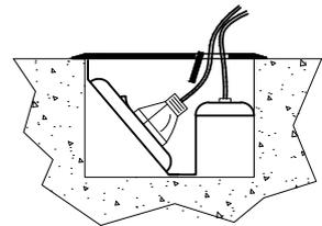
ASSEMBLED SIDE VIEW OF FB147 TWO COMPARTMENT FLOOR BOX SHOWING CABLE EXIT FLAP IN USE
